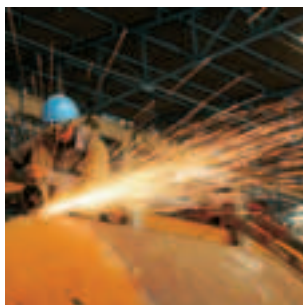
Finishing operations of Washer Drum.
