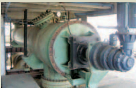
Continuous Digester at Naini Papers, Uttaranchal.
