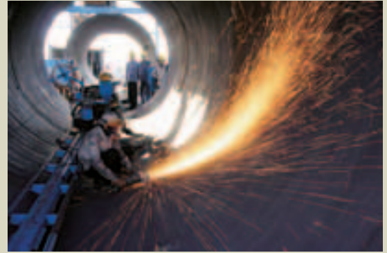
Manufacture of MS Pipes of 300 mm to 2350 mm dia at site for Narmada Irrigation Pipeline Projects in Gujarat.
